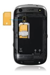
Slide the SIM card into the slot.
