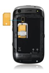
Slide the SIM card into the slot.
