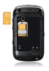
Slide the SIM card into the slot.
